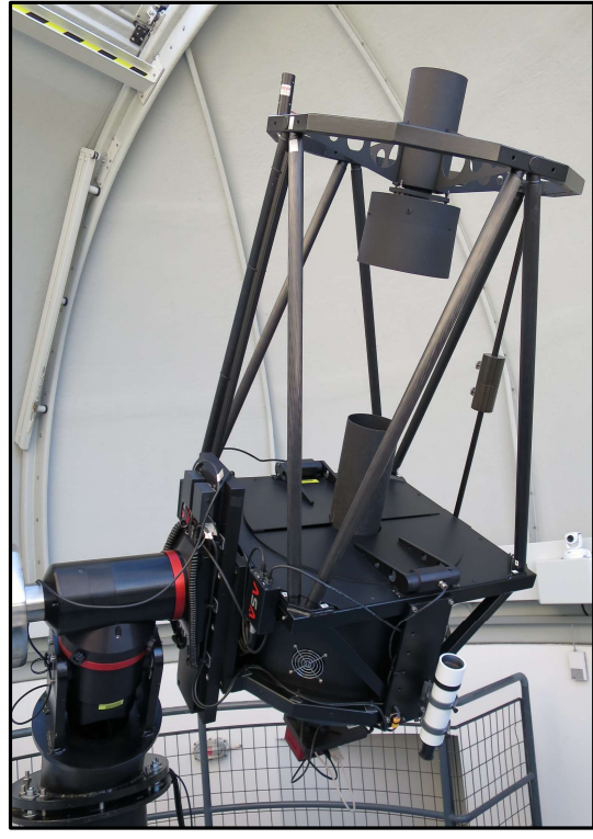
ASA 50 cm Cassegrain telescope (f/9)
